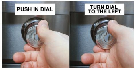
Turning the dial (see left photo - overhead perspective) counter-clockwise a quarter turn will fire the ignitor contact within the cabinet (see arrow). (For a wide-shot view of the entire griddle from an overhead perspective, refer to the right hand side photo.)
