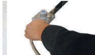
**After orifice has been tightened attach flexible hose**
