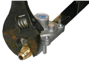
**Use a wrench to tighten down the orifice**
