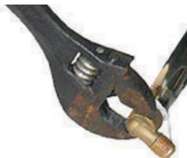
Turn propane valve counter-clockwise to loosen
