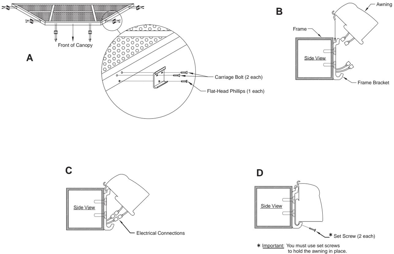
**Figure 39.** Awning Installation
