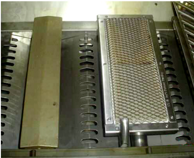
One infrared burner installed
