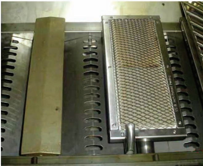
One infrared burner installed
